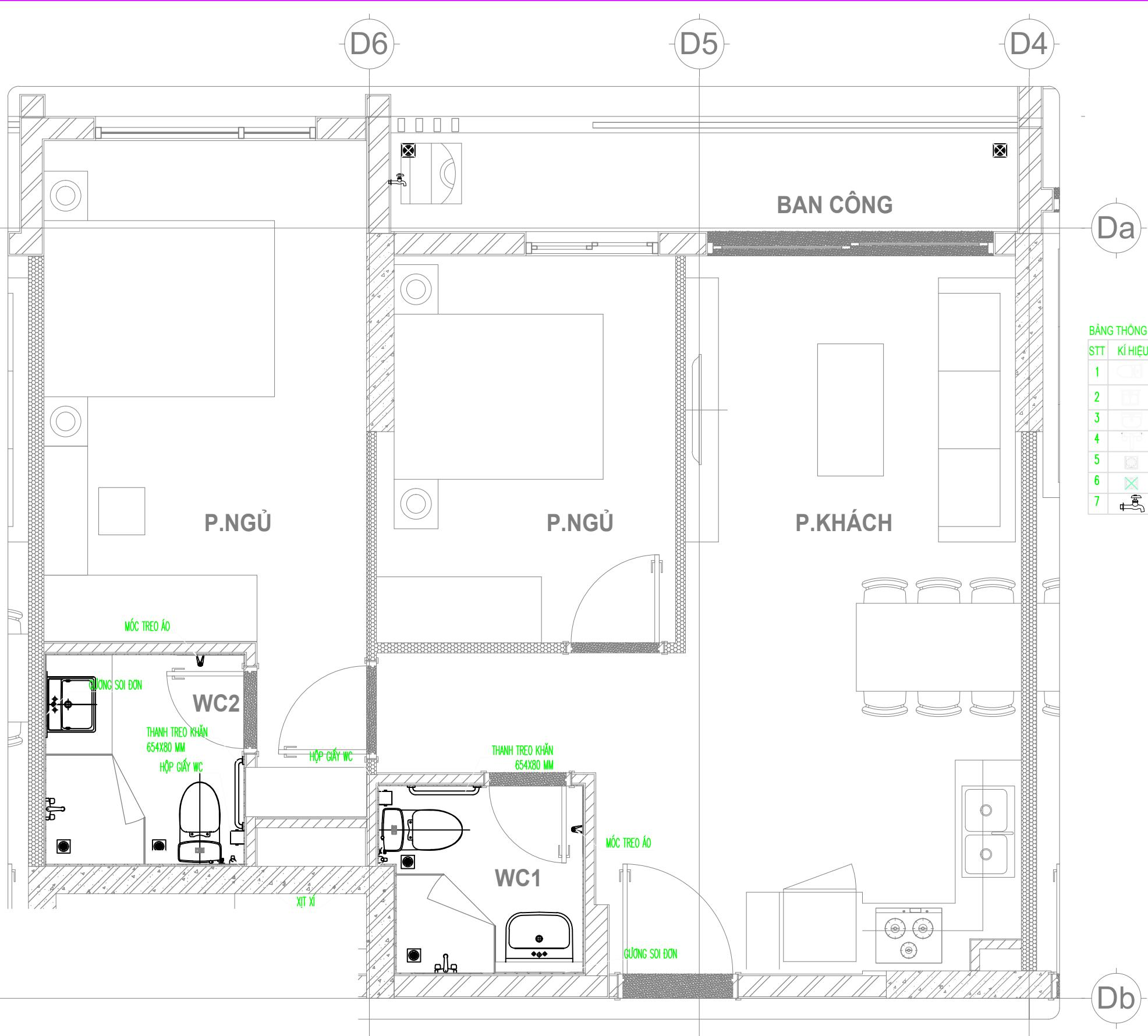
MẶT BẰNG LẮP ĐẶT THIẾT BỊ VỆ SINH CĂN HỘ D2-xx-07/140
