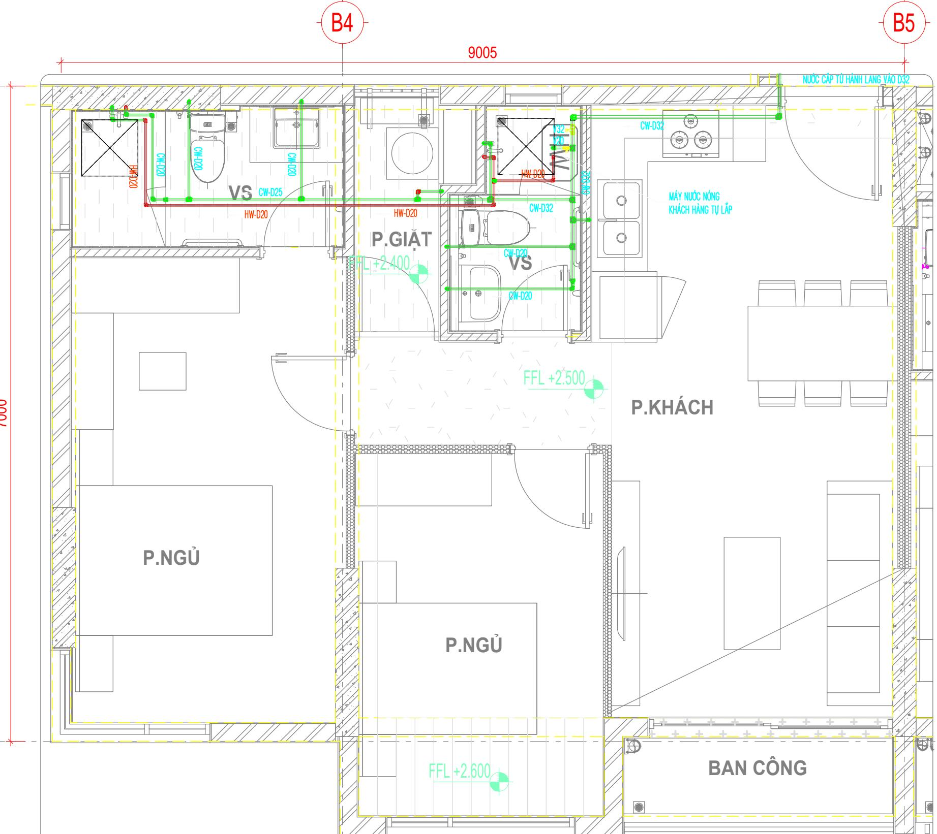
MẶT BẰNG CẤP NƯỚC CĂN HỘ B2.(3-21).11
