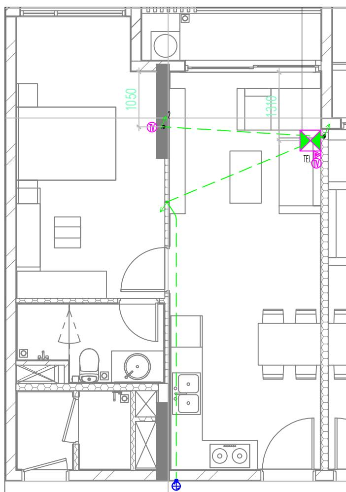
MẶT BẰNG HỆ THỐNG ĐIỆN NHẸ CĂN HỘ B2.(03:21).07
