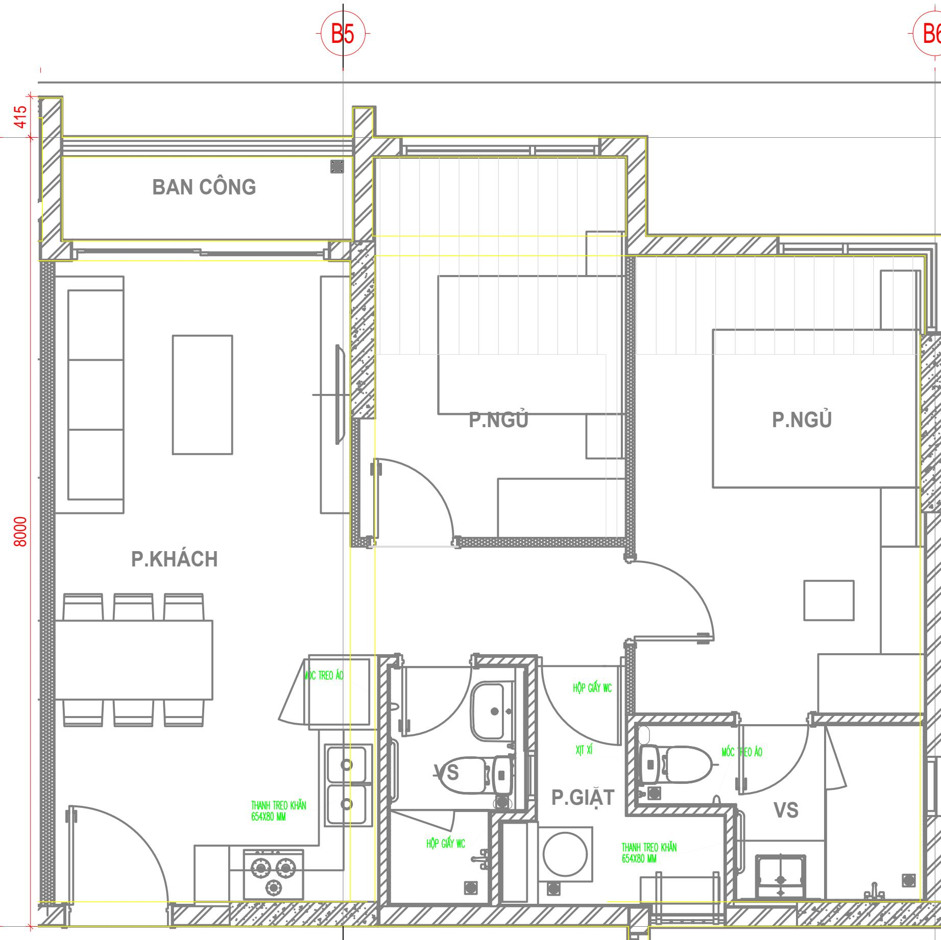
MẶT BẰNG LẮP ĐẶT THIẾT BỊ VỆ SINH CĂN HỘ B2.(3-21).06
