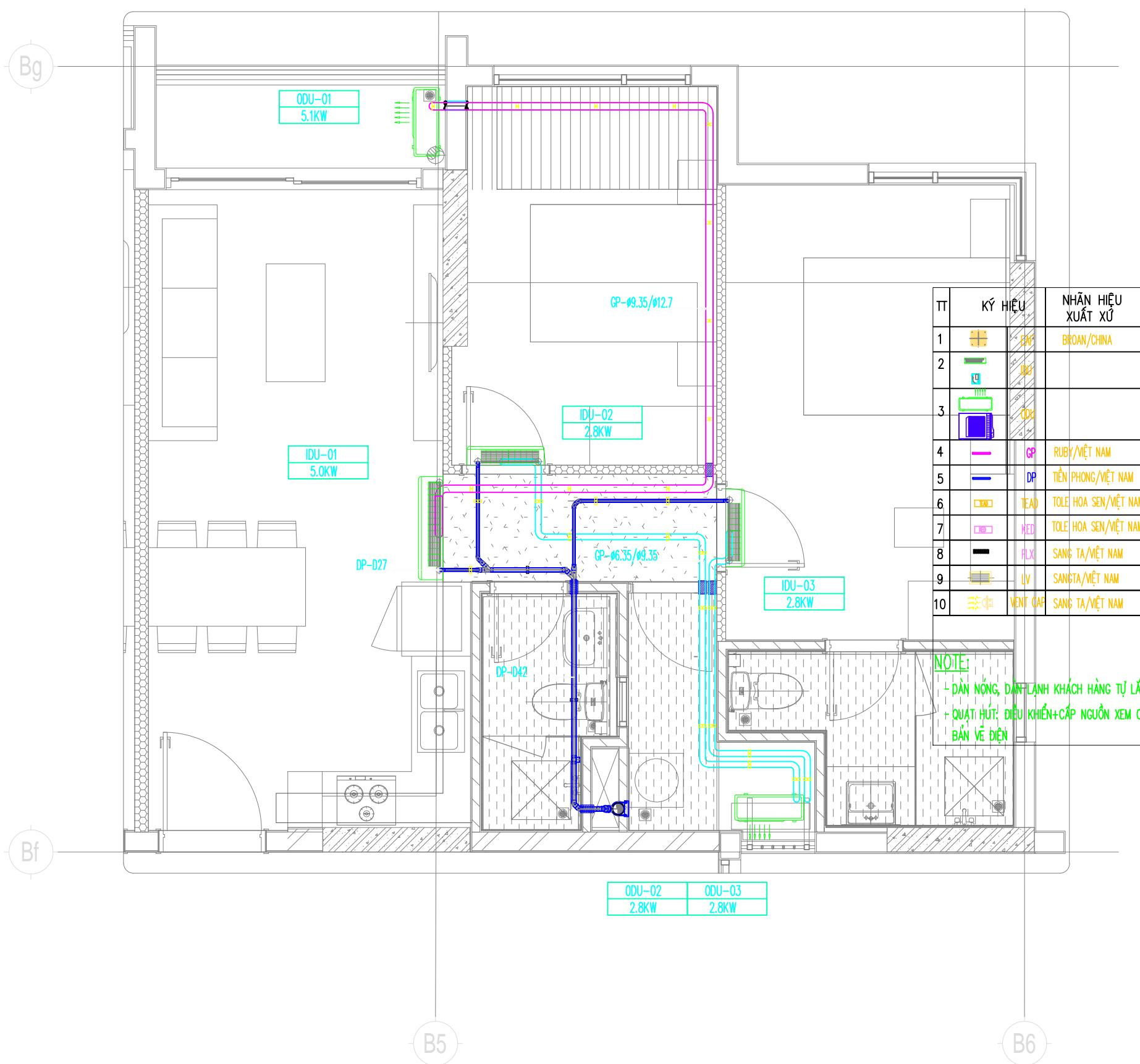
01 MẶT BẰNG HỆ THỐNG ĐIỀU HÒA KHÔNG KHÍ CĂN HỘ SỐ B2.\*\*.06-THÁP B
