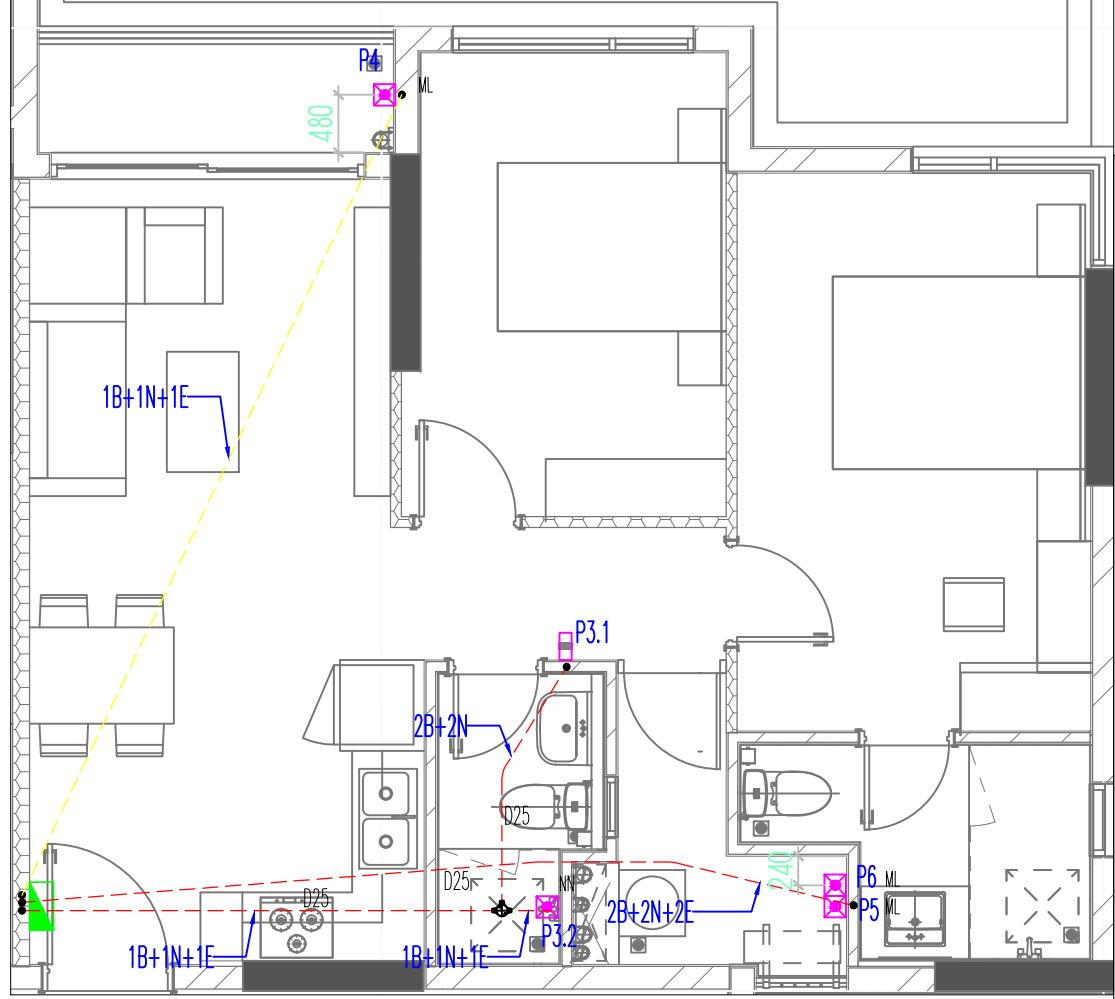
MẶT BẰNG KÉO DÂY CẤP NGUỒN CĂN HỘ B2.(3:21).06
