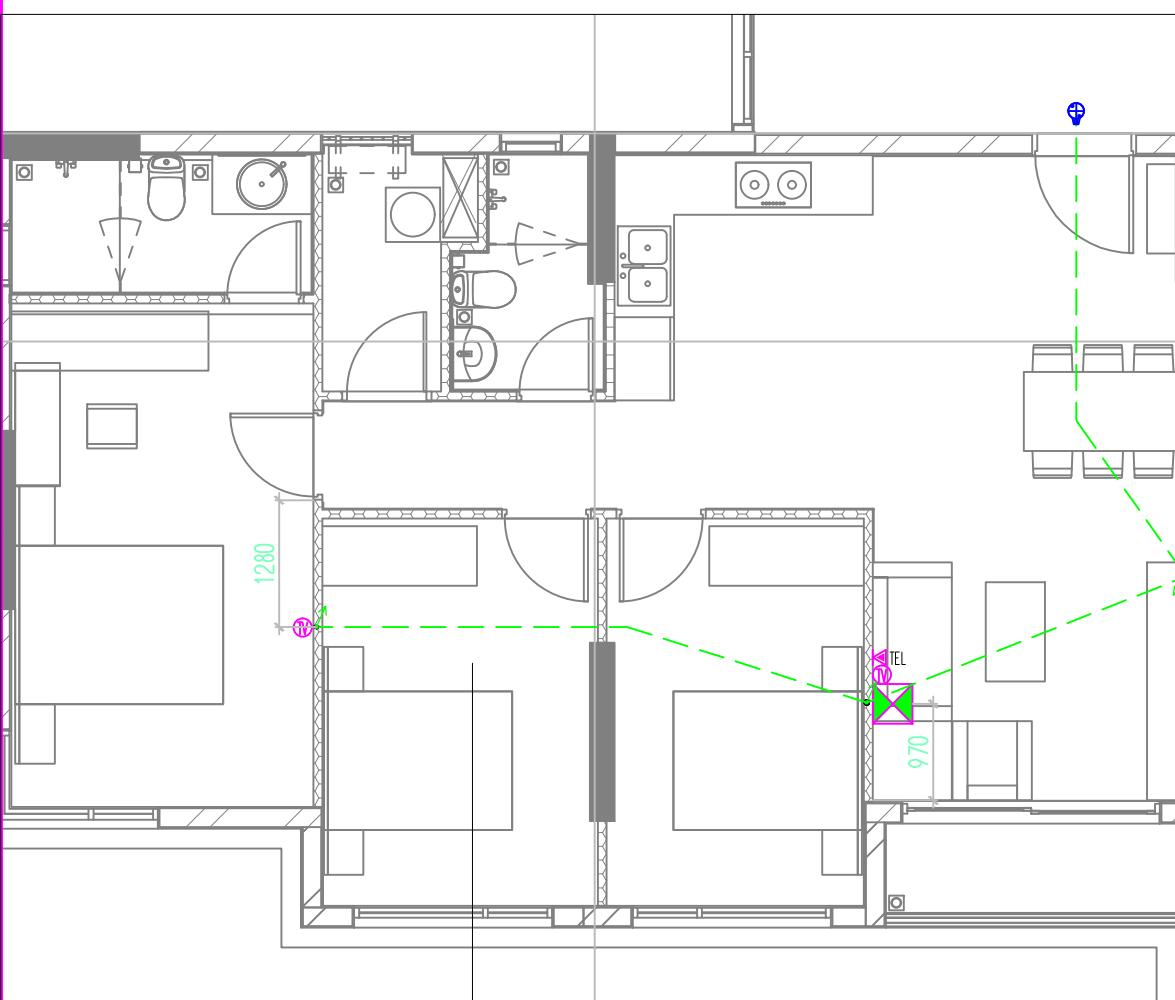
MẶT BẰNG HỆ THỐNG ĐIỆN NHẸ CĂN HỘ B2.(03:21).02
