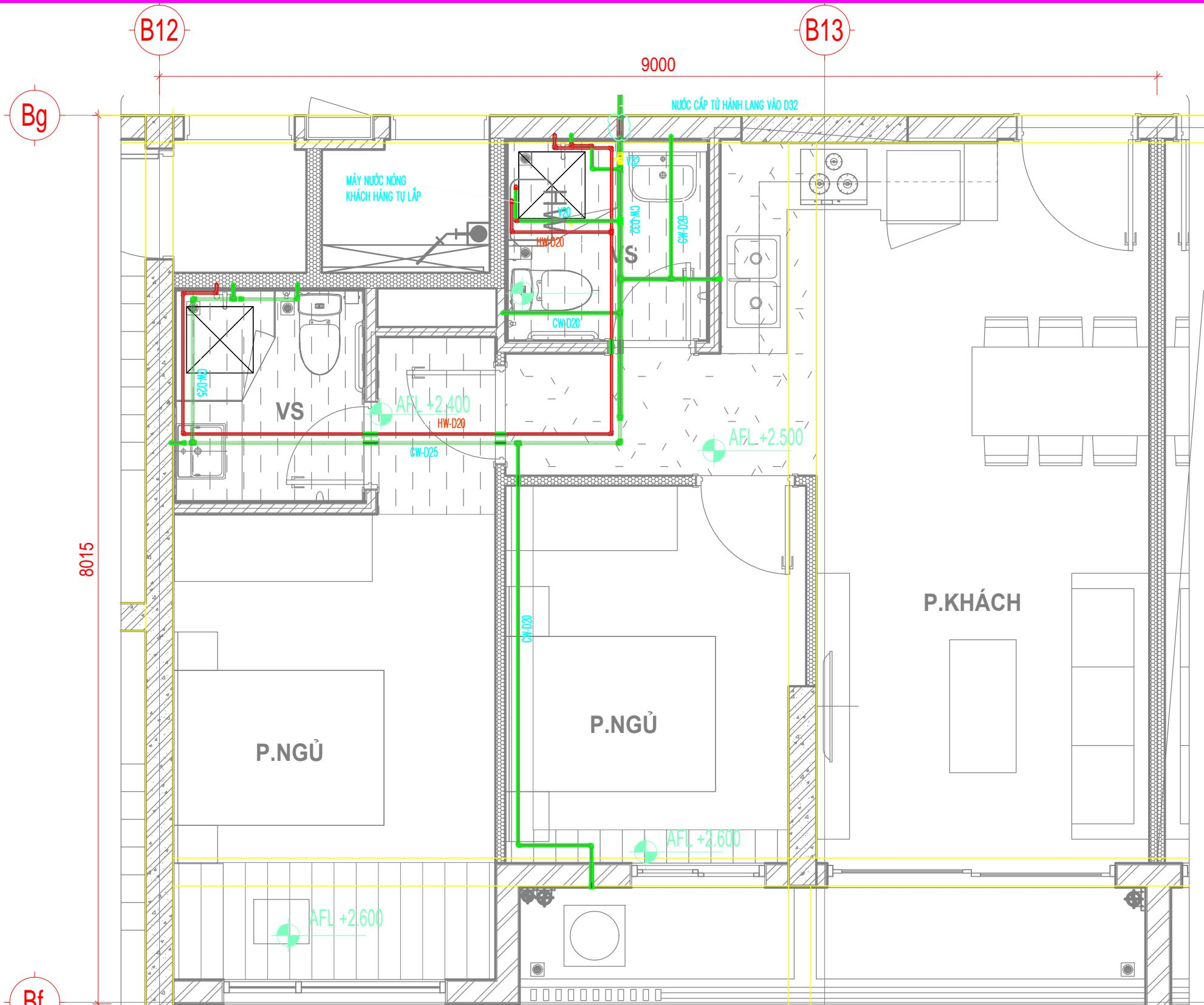
MẶT BẰNG CẤP NƯỚC CĂN HỘ B1.(3-21).10
