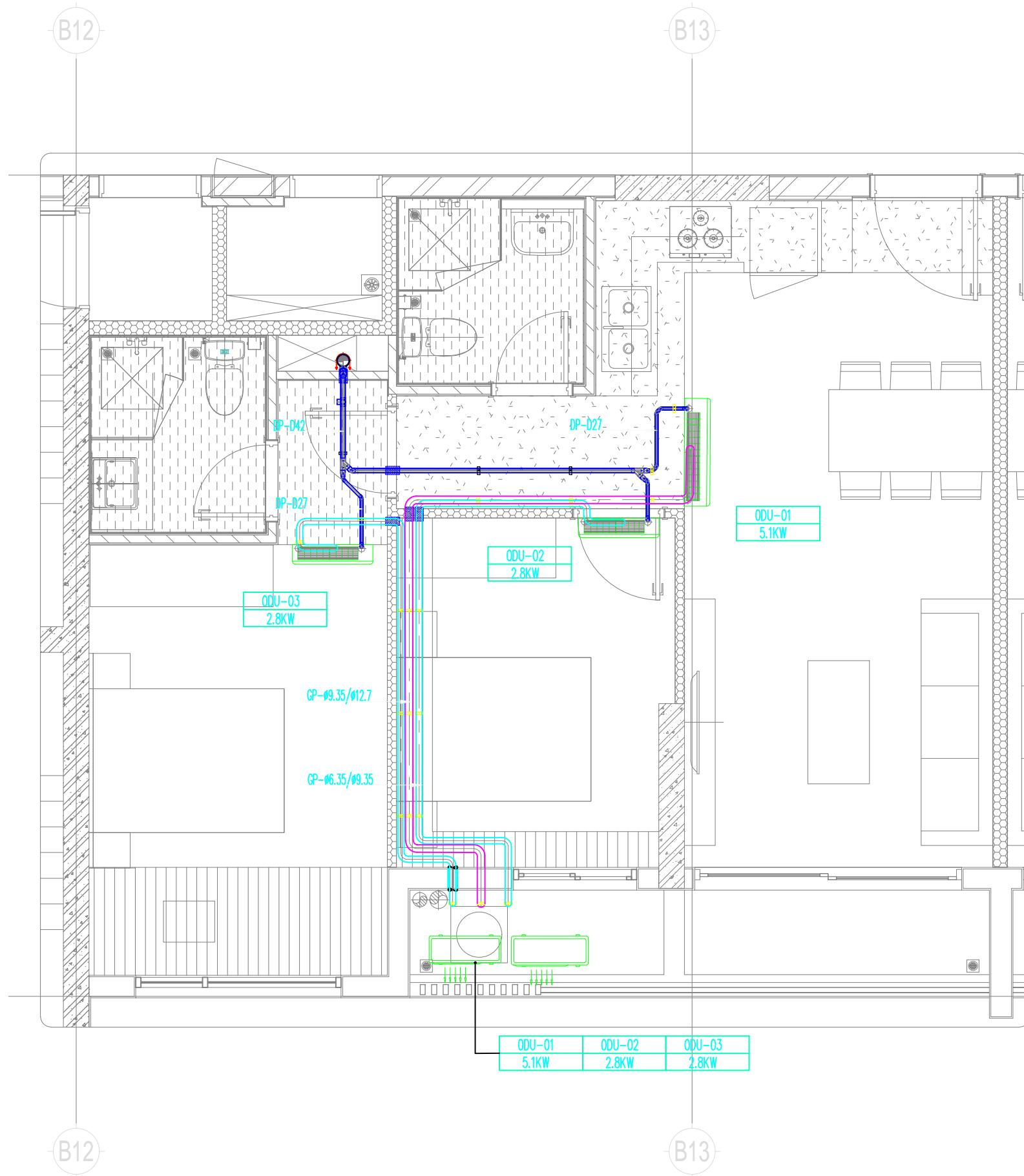
01 MẶT BẰNG HỆ THỐNG ĐIỀU HÒA KHÔNG KHÍ CĂN HỘ SỐ B1.\*\*.10-THÁP B
