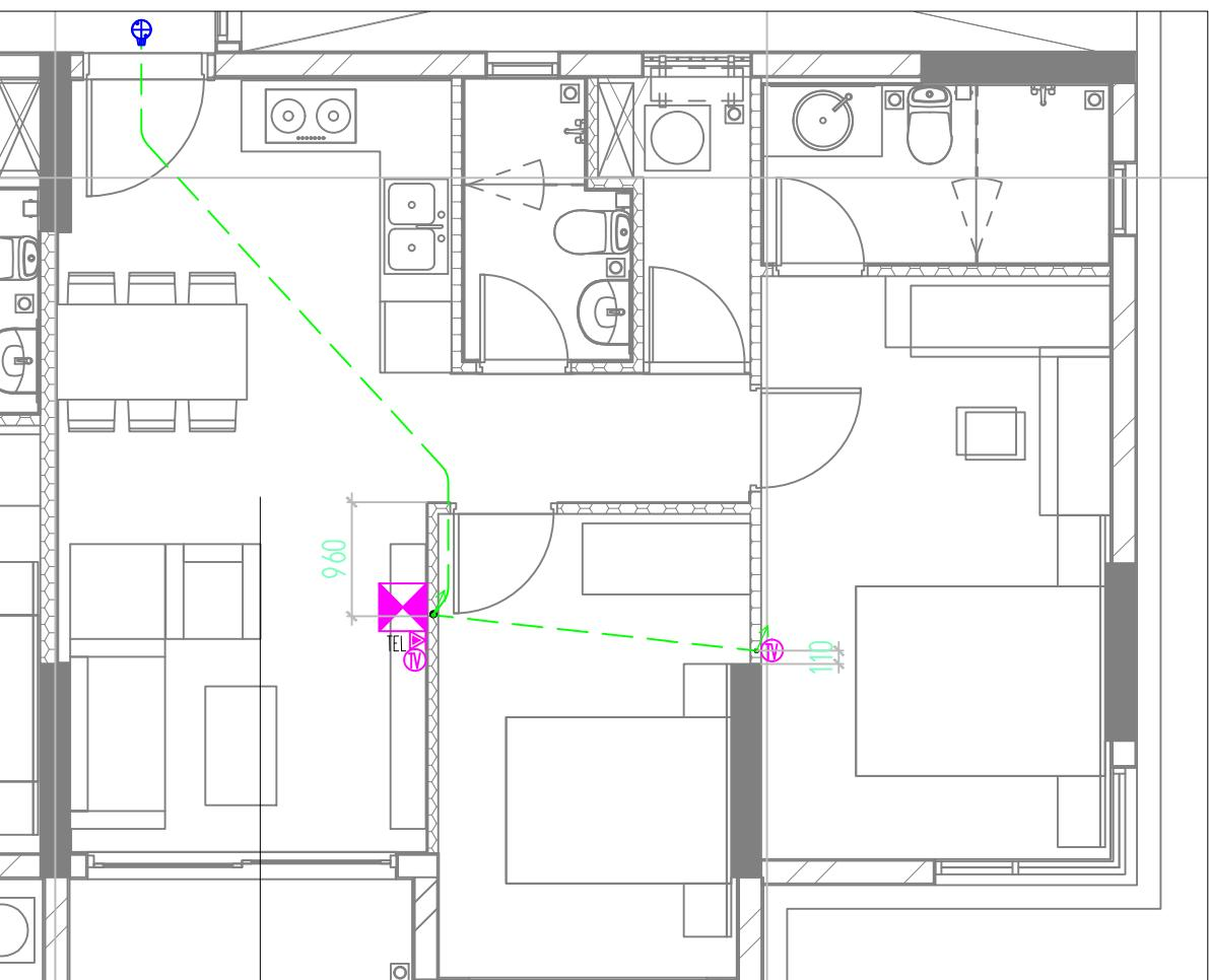
MẶT BẰNG HỆ THỐNG ĐIỆN NHẸ CĂN HỘ B1.(03:21).01
