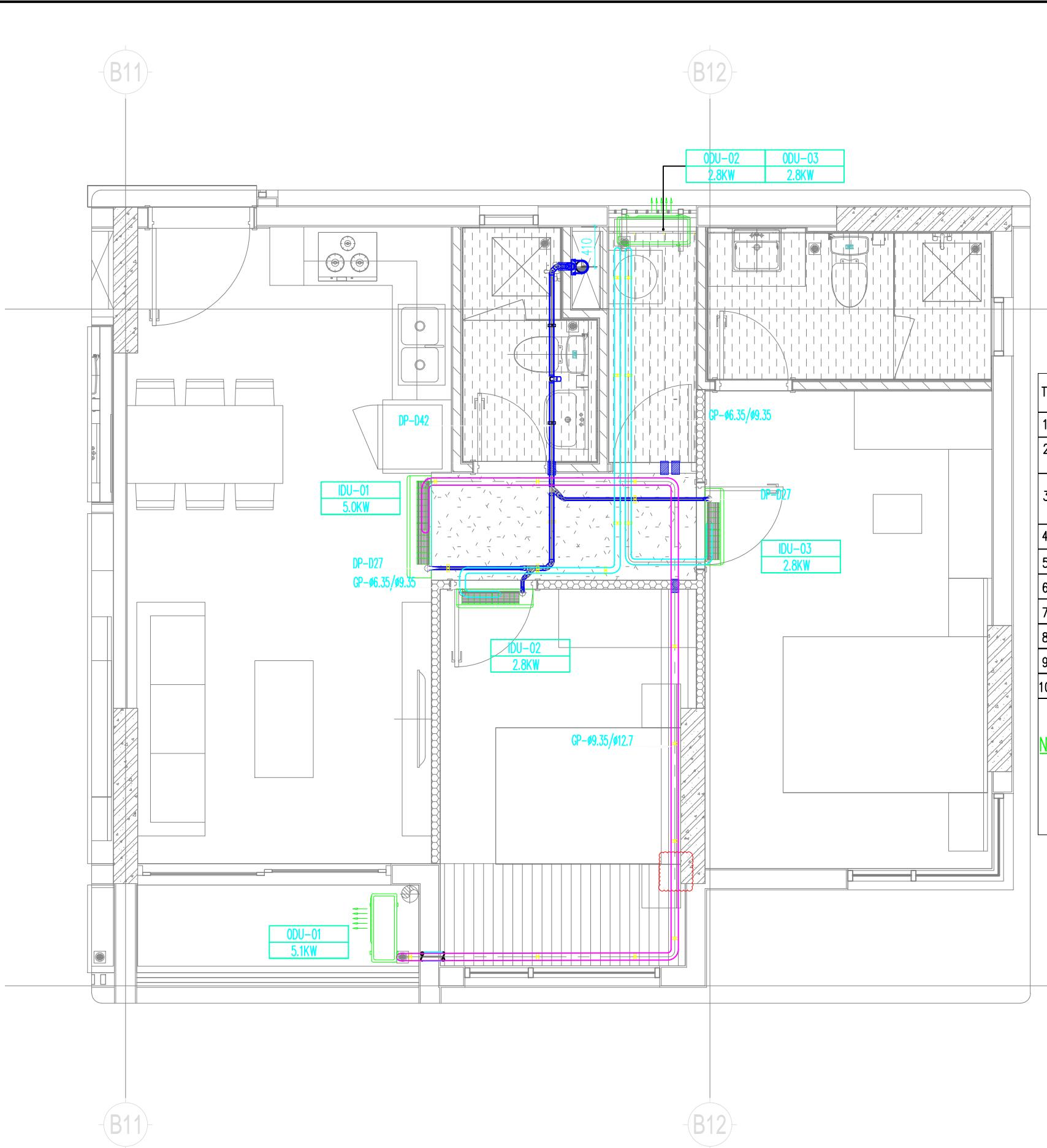
01 MẶT BẰNG HỆ THỐNG ĐIỀU HÒA KHÔNG KHÍ CĂN HỘ SỐ B1.\*\*.01-THÁP B
