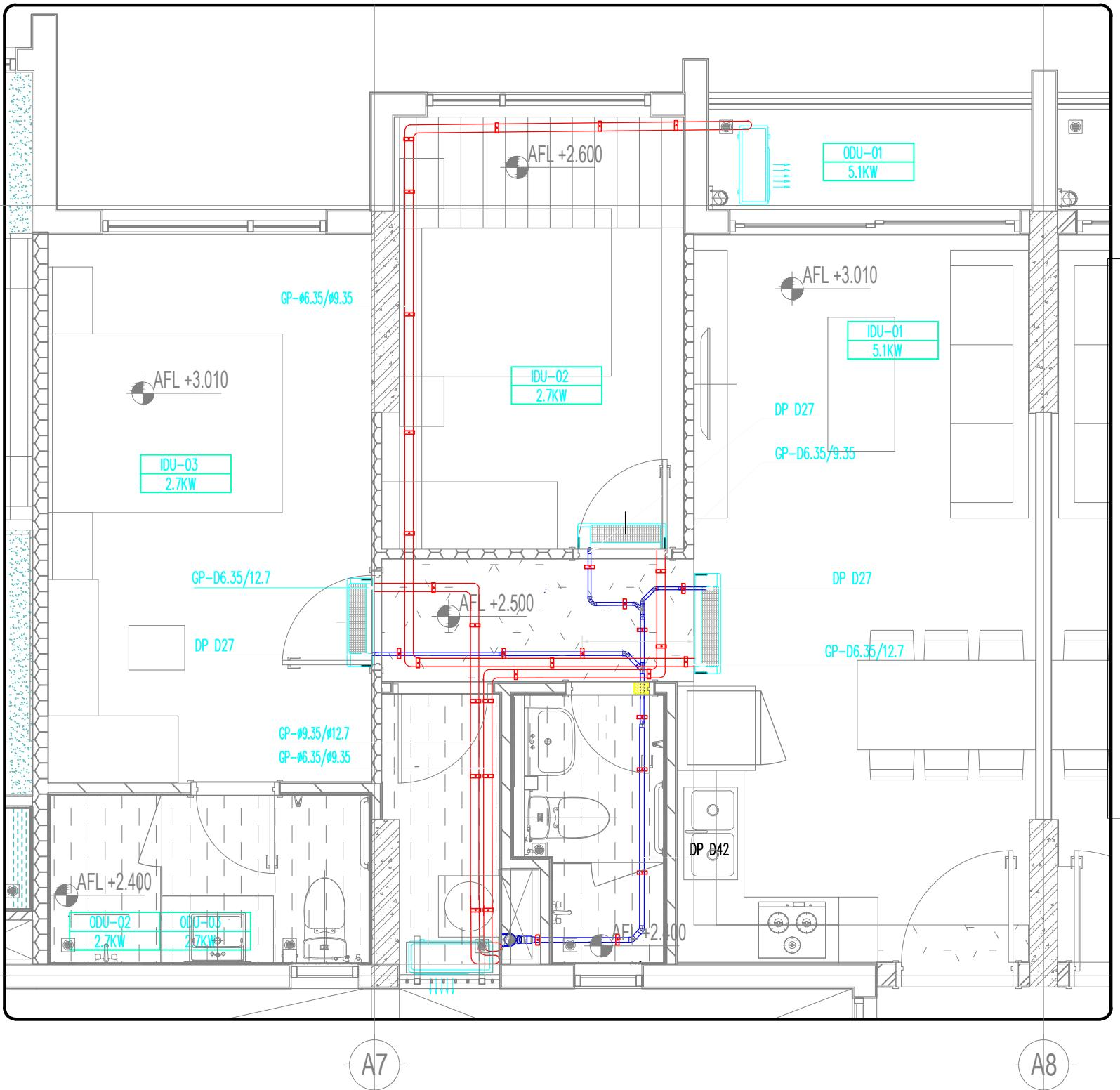
01 MẶT BẰNG HỆ THỐNG ĐIỀU HÒA KHÔNG KHÍ CĂN HỘ SỐ A2.\*\*.07-THÁP A
