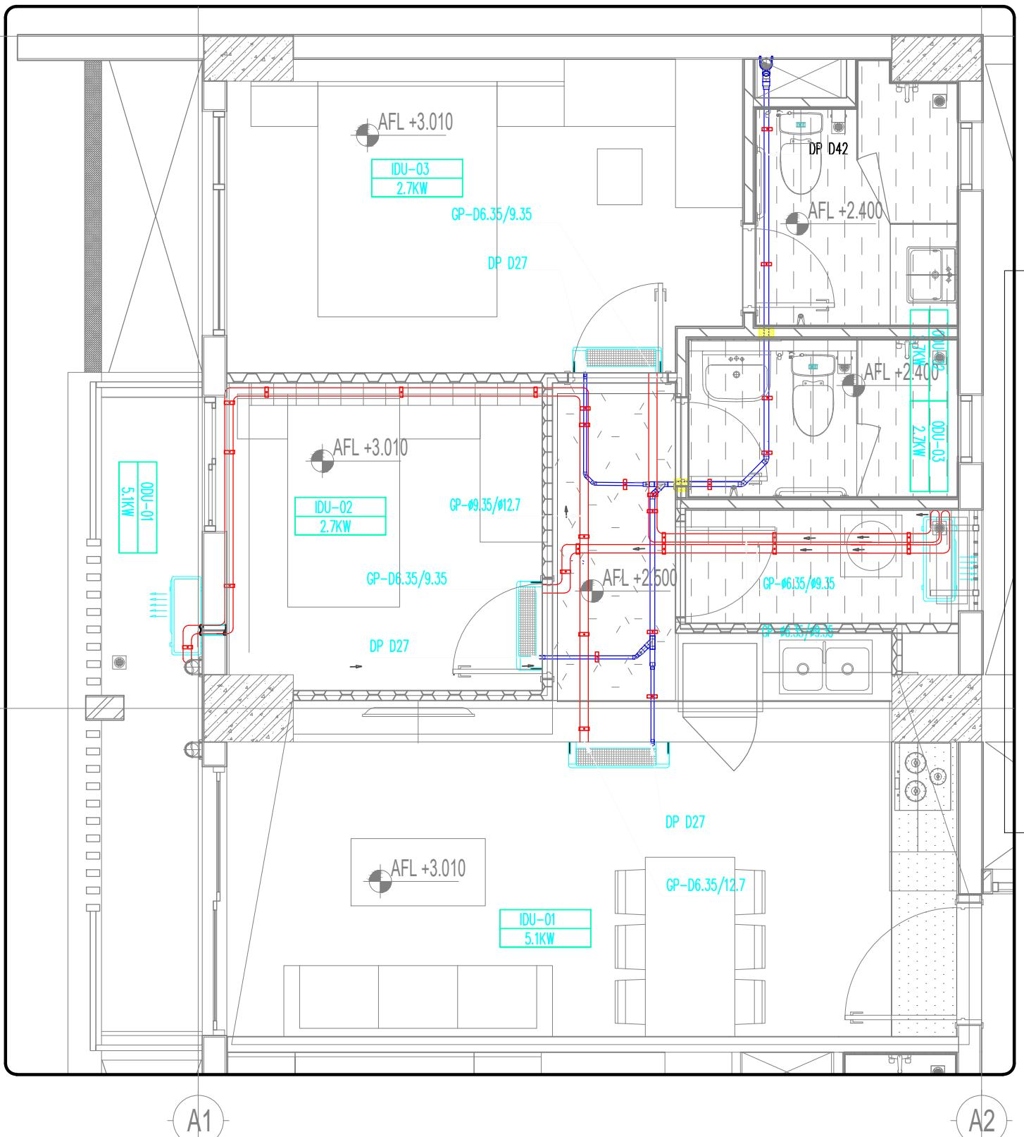
01 MẶT BẰNG HỆ THỐNG ĐIỀU HÒA KHÔNG KHÍ CĂN HỘ SỐ A1.\*\*.08-THÁP A
