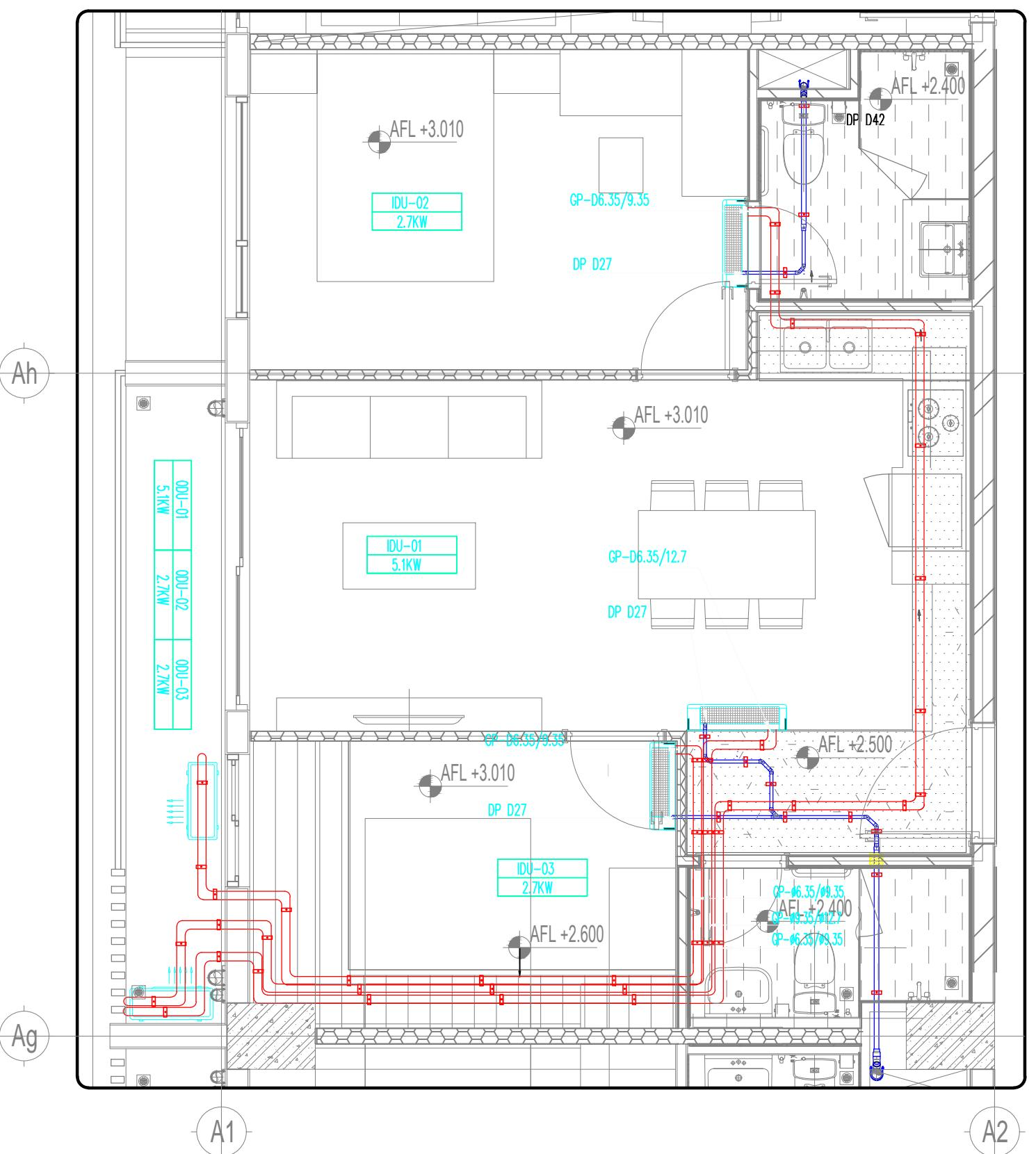
01 MẶT BẰNG HỆ THỐNG ĐIỀU HÒA KHÔNG KHÍ CĂN HỘ SỐ A1.\*\*.07-THÁP A
